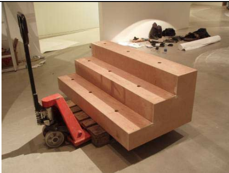
(a) The staircase used for the UFO-installation. Nine holes ensure inputs from nine pressure sensors.
