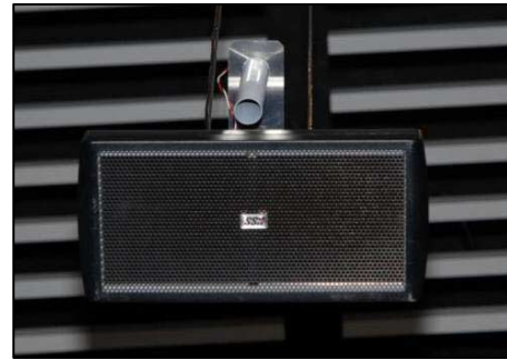
Figure 2: The directional speaker and a PIR sensor shielded in a tube four meters above the floor.
